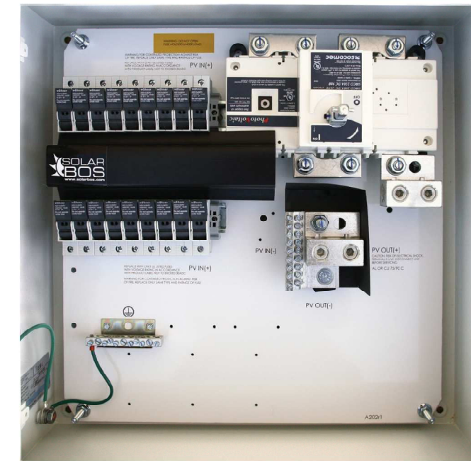
SolarBOS Disconnect Combiner, 1000VDC, 250A disconnect switch, 18 input circuits, dual output lugs, NEMA-4 powder coated steel enclosure
